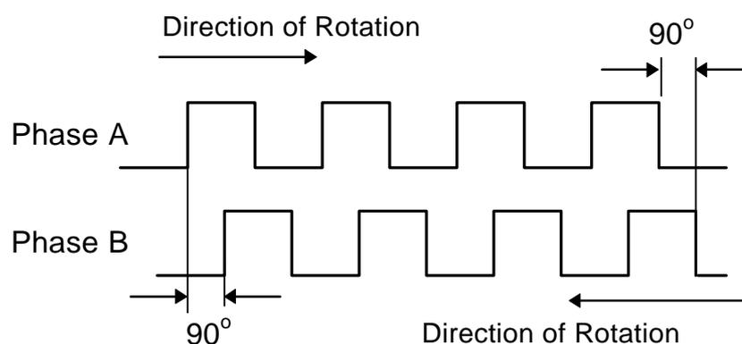
When the encoder shaft rotates in one direction, phase A leads phase B by 90 degrees. When the shaft rotates in the opposite direction, phase B will lead phase A by 90 degrees. The quadrature signals therefore provide an indication of the direction of rotation.
