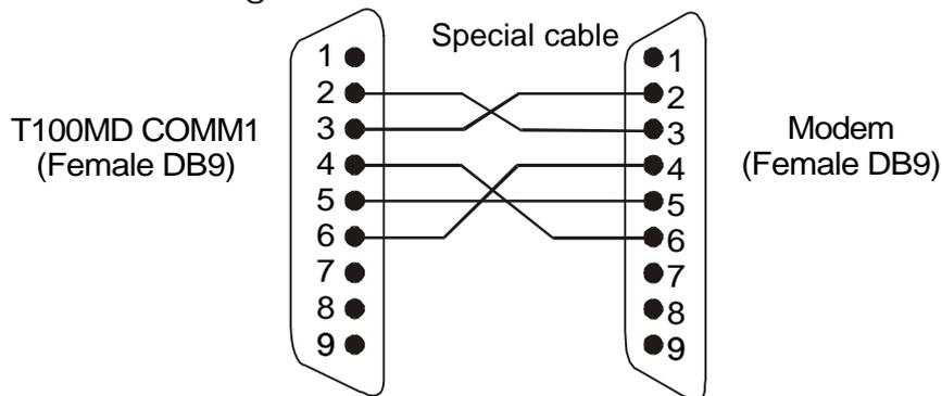
Figure 1.10 Connecting COMM1 to a MODEM
