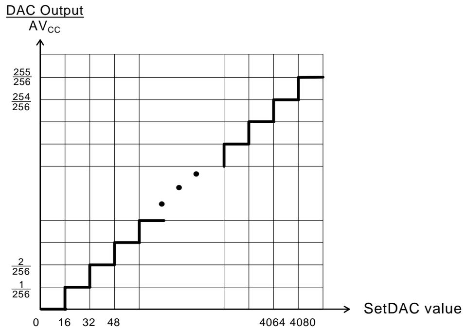
Figure 1.8 Transfer Function for 8-bit DAC.
