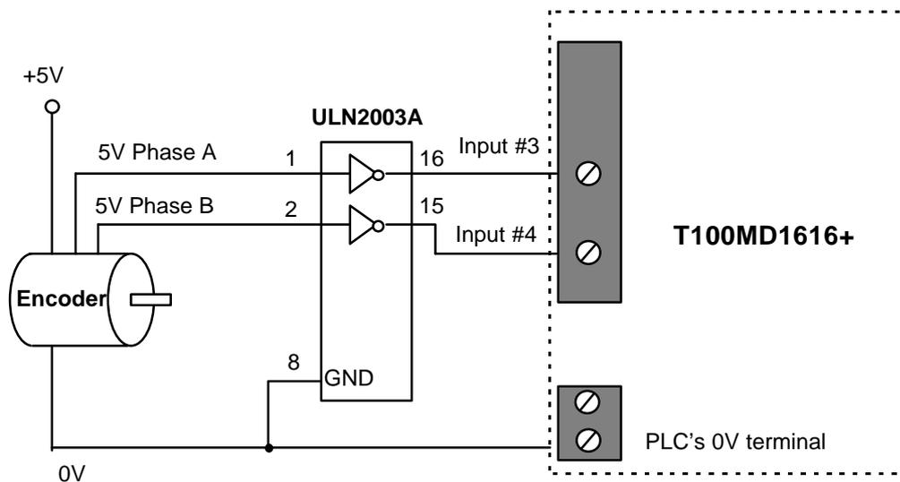
Figure 1.5 Interfacing 5V type Rotary Encoder
