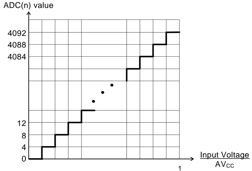
Figure 1.7 Transfer Function for 10-bit ADC.
